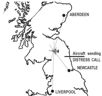
Fig 4-9: How triangulation is used to locate aircraft in distress
