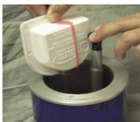
Fig. 8 Place container on the wax injector so the teeth side of the denture is injected first.
