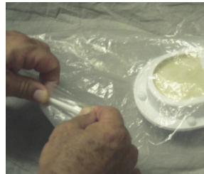
Fig. 6 Place top onto container, place into resealable plastic bag and seal bag.
